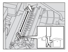
12 Return the transfer charger cleaner into the cleaner pocket, and then close the transfer unit.
